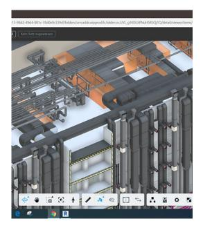
A CDE (common data environment) is used to manage the BIM models, the BIM documents, and other relevant BIM planning data. The environment enables around 80 participants to work on a shared BIM data model via multiple authorisation levels, while complying with extensive data protection requirements.
